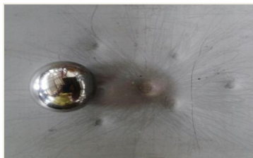
▷ Plate surface is crushed after vertical vibration
