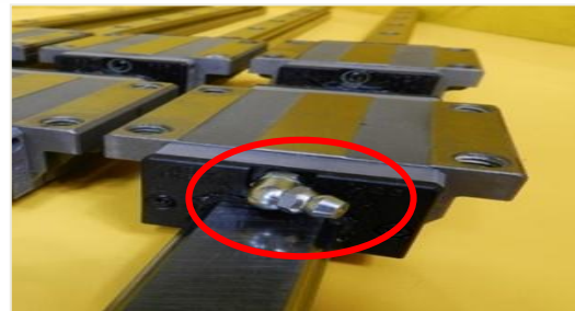
(Lubricating oil injection)
