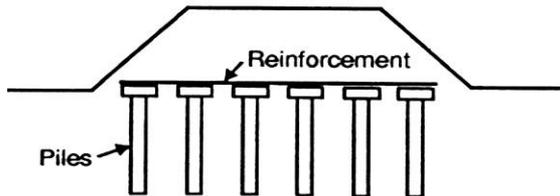
e) Basal reinforced piled embankments
