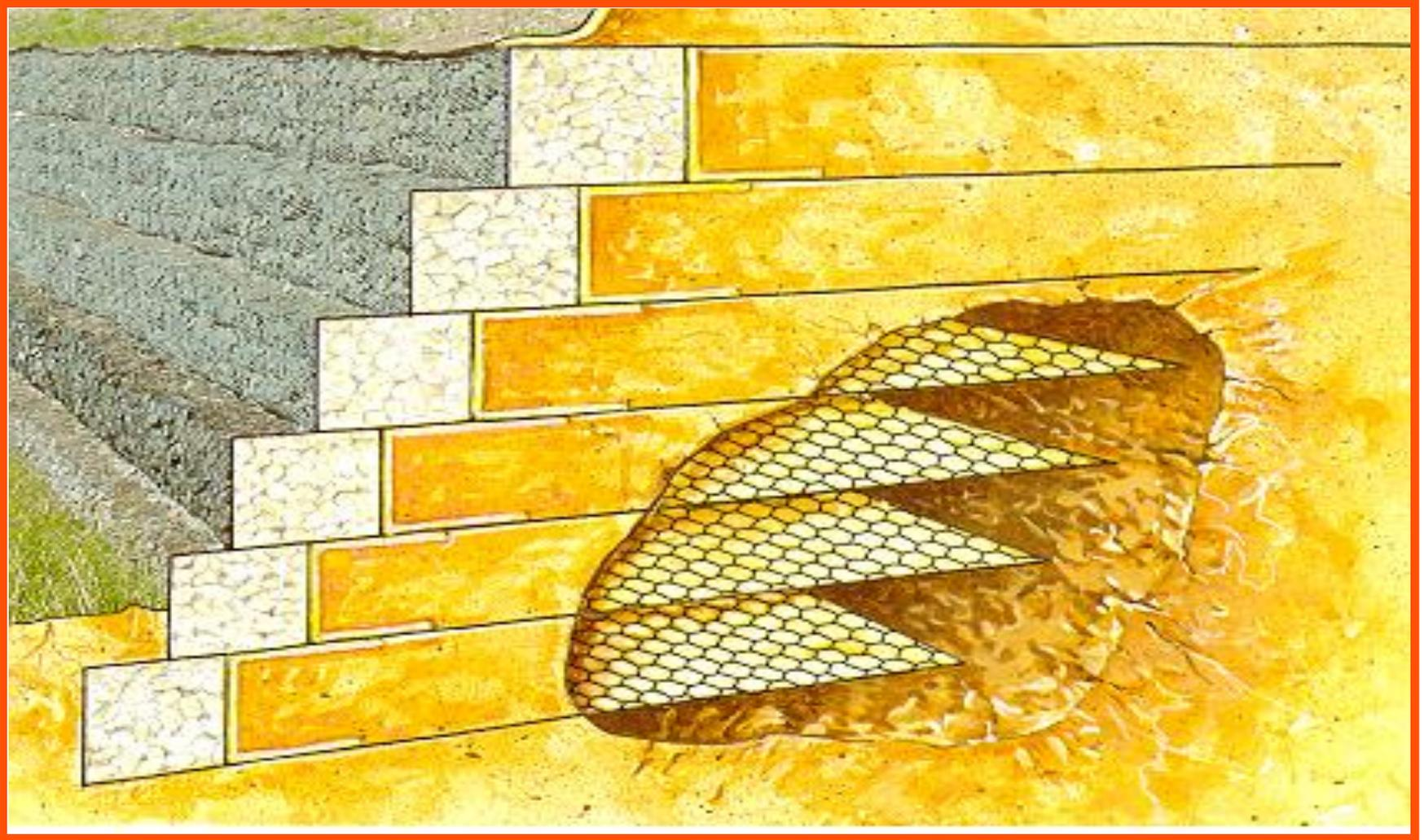
**Reinforced Soil Structures: Terramesh System**
