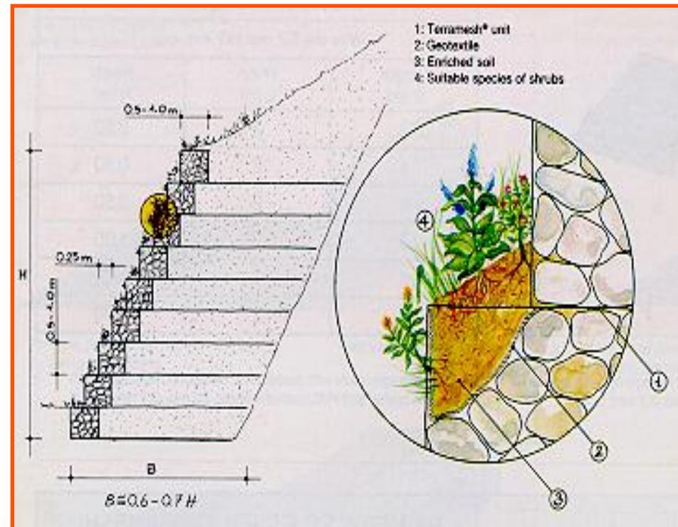
Green Terramesh<sup>®</sup> System - Similar to the other Terramesh but without the gabion type face, its external surface is always inclined and it is made using hexagonal netting with a structural function and with bio-degradable mat to retain soil particles and also to help grow vegetation.
