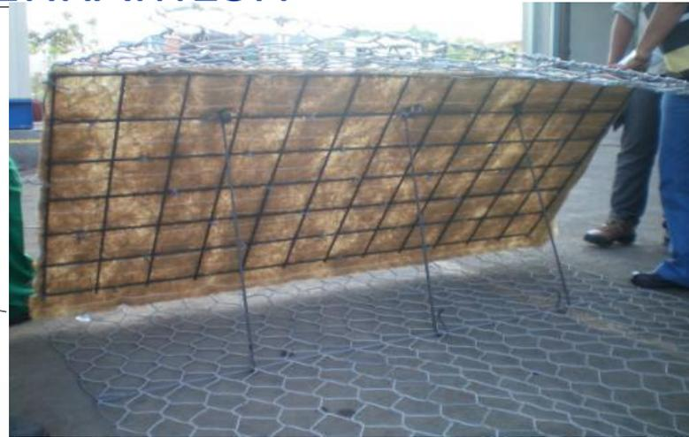
Terramesh<sup>®</sup> System - Structure consisting of an external face, stone filled gabion type, continued as a double twist mesh panel, both PVC coated. They can be built with a stepped or vertical face, with or without a batter.
