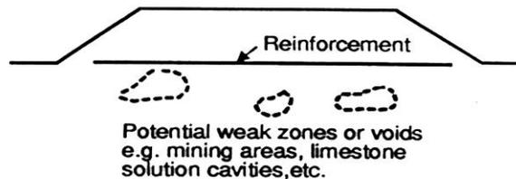
f) Basal reinforcement spanning voids
