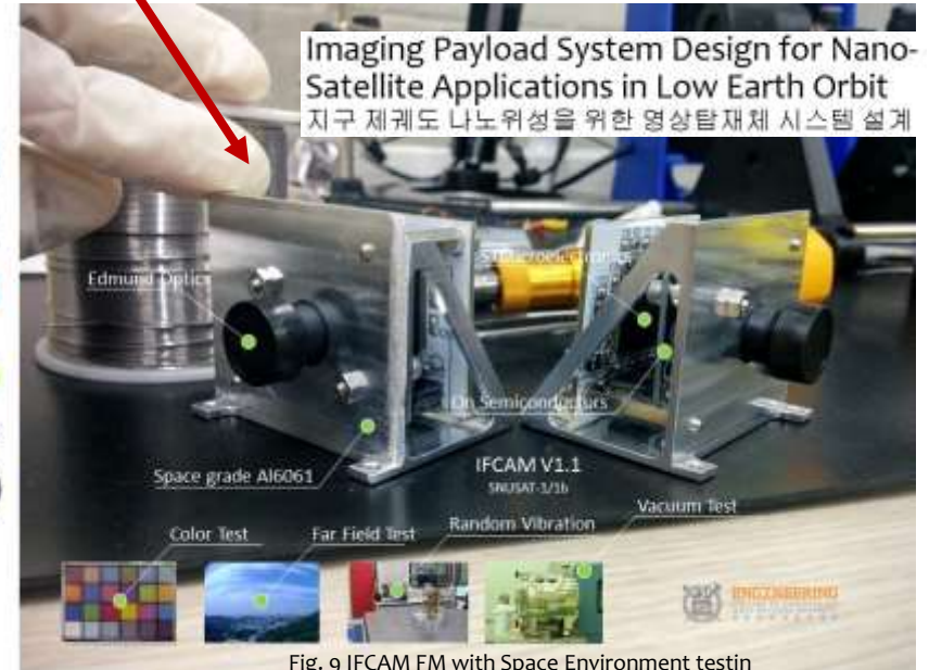
Fig. 9 IFCAM FM with Space Environment testin g [Photo by Maskey, 2016]
